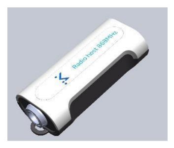
ML RF Host -868 Needed for SDI for communication with ML Timing gates. NB! DSU has built in RF Host-868 Communicates with up to 10 Timing gates simultaneously
