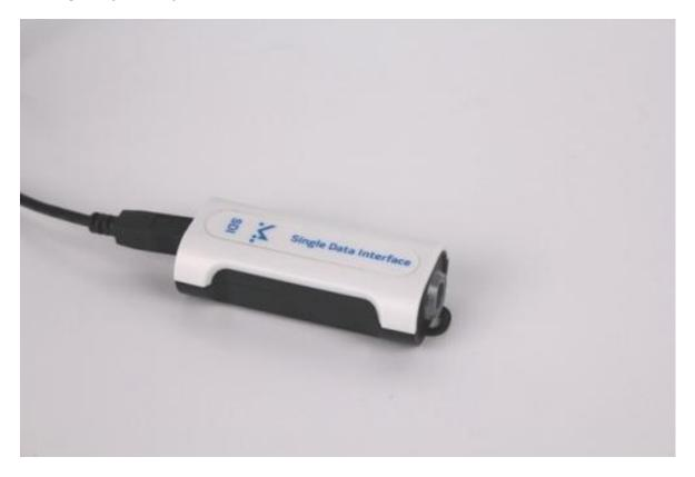
**SDI** – is short for "Single **D**ata Interface" and is a simpler version of the **DSU**. The SDI has only one port for connection for sensors or accessories.
